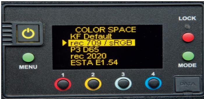
**Color Space** defines the RGB color space used and only affects color – not Kelvin. It is used in **RGB** mode and **Hue Angle** and **Saturation**. There are a few instances in the FX (Effects) mode that are also affected when color is used. The RGB color space defines the value of Red, Green, and Blue primaries (in CIE xy) and the white point is fixed at 6500 Kelvin. Exception being **ESTA E1.54** which is a fixed point at 3200 Kelvin.
