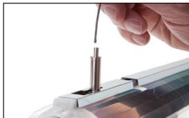
Insert into T-slot. Insert wire all the way down. Pull up wire until it latches. Press down pin to release wire.
