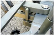
Switch lever (here in upward position)
