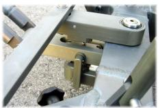
Switch lever (here in the downward position)
