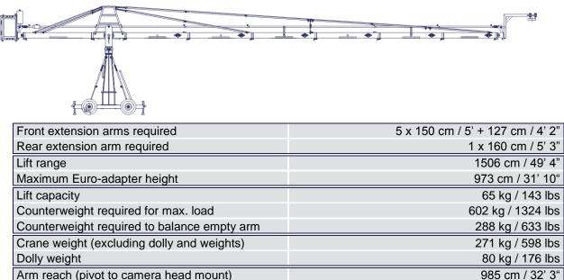
Double rigging is required! Observe guidelines on page 43 and additionally ensure that the Large Rigging Harness is used with double rigging to the rear and front.
