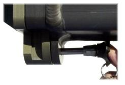
Securing the arm with a safety pin
