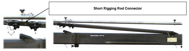
6. After the complete rigging system has been assembled, hand tighten the turnbuckles until the rigging rods are taut. The turnbuckles can be secured with locking nuts. Make sure that the rigging is absolutely straight. For this case the Adjustable Rigging Rod Support has to be adjusted in a proper way.
