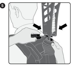
Adjust according to your height To raise the upper arm further, release the two screws on the upper block (under the rubber bellow).
