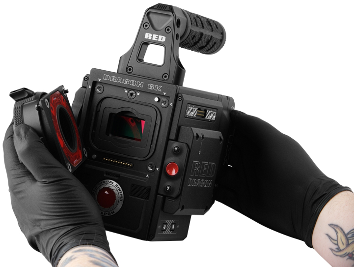
Figure: Remove the Lens Mount
