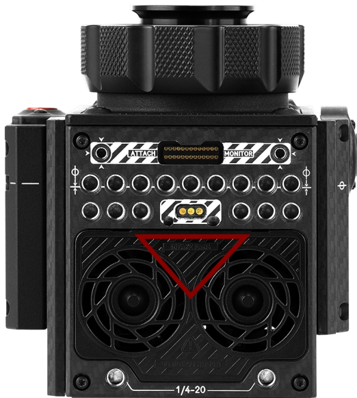
Figure: Do Not Obstruct WiFi Antenna
