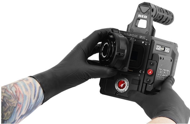
Figure: Align Lens Mount Pins
