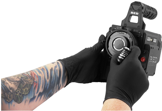
Figure: Remove the Lens Mount Screws
