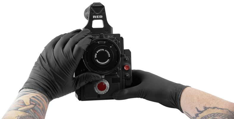
Figure: Turn Locking Ring Counter-Clockwise
